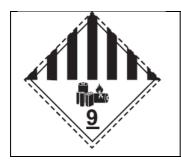
**Symbol** – seven vertical bars in black in the upper half **Background** – in white color (battery group, one broken and emitting flame) **Number 9** – In the bottom corner
