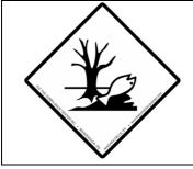
Packages and cargo transport units containing dangerous substances which are classified by the IMDG Code as "marine pollutants", must have the markings shown here, which must be durable. They must be placed close to the risk labels or risk placards of the goods. The dimensions of the marine pollutant markings must be a minimum of 10 cm per side for packages and 25 cm per side for cargo transport units.
